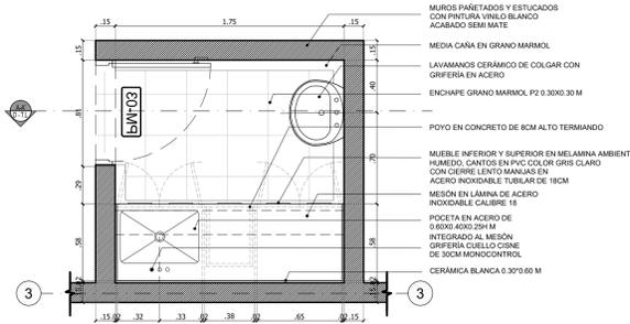
DETALLE TRABAJO LIMPIO / D-T-L / PLANTA ESC.....1:25
