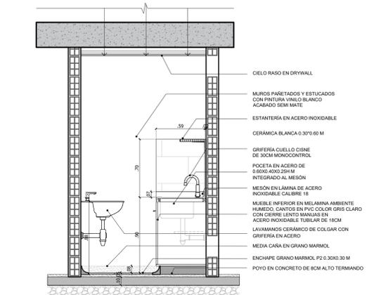
DETALLE TRABAJO SUCIO / D-T-S / A-A' ESC.....1:25
