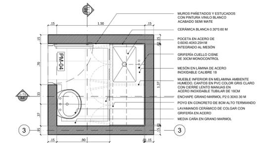
DETALLE TRABAJO SUCIO / D-T-S / PLANTA ESC.....1:25
